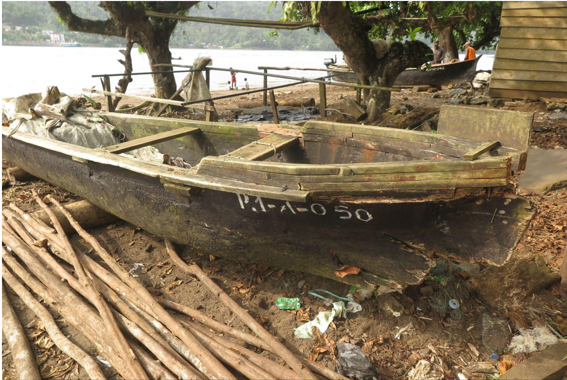
Fig 6. Detail photo of several wooden strips placed on top of each other for the purpose of increasing the load capacity of the canoe, in Santo António do Príncipe. (Photo: G.L.)
