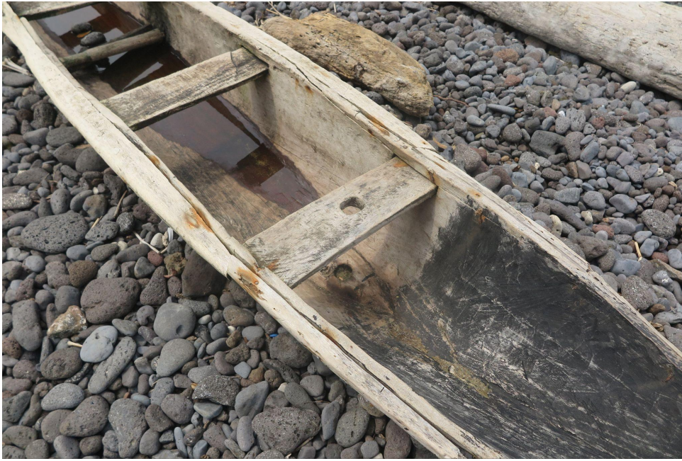
Fig 7. Detail photo where the system of hoisting the mast of a dugout canoe can be observed. (Photo: J.B)
